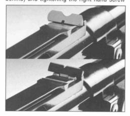
the bead moves to the left and the point of aim on the target to the right (1 mm = approx. 20 cm/100 m, 1/32" = approx. 8"/110 yd.).
