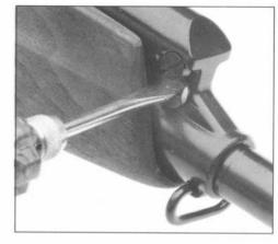
The hole in the plug is dimensioned so that the rifle operates perfectly using factory-made cartridges with bullet weights of 10 - 14 g (150 - 210 grs). If you make up your own cartridges or use factory-made cartridges with a lighter bullet weight, ask your dealer for a substitute gas plug (optional).
